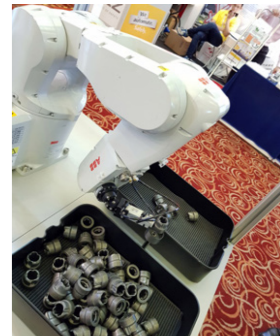
Robotic bin picking in action.
